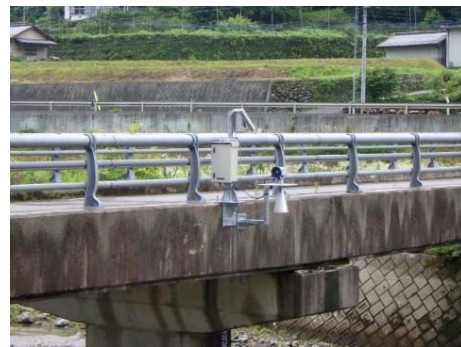
Crisis-management type water gauge (low-cost water gauge specializing in water level monitoring during floods)
